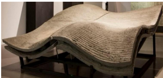
Figure 3: Curved Concrete Plate Made Using Additive Manufacturing
