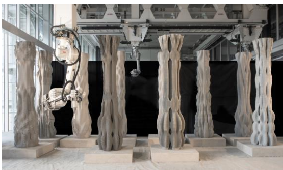
Figure 13: Concrete Pillars Made using Additive Manufacturing
